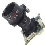
FWC-EE1-307 — 2MP rolling-shutter single-board module (Eyenix).
